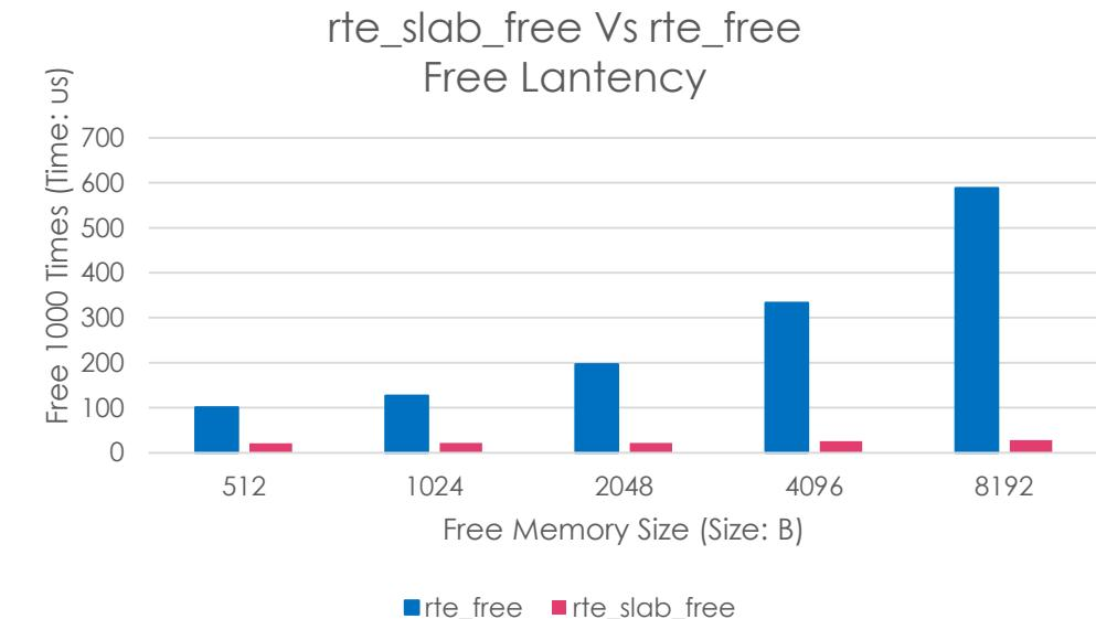
rte\_slab\_malloc better than rte\_malloc: 75%
