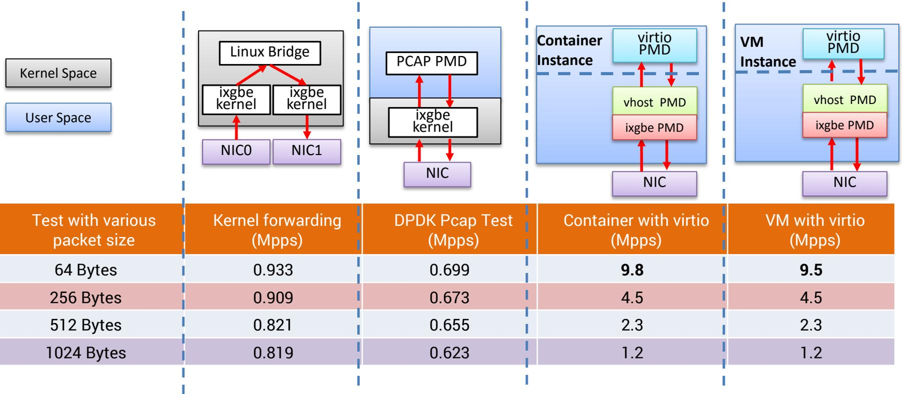
CPU: Intel(R) Xeon(R) CPU E5-2699 v3 @ 2.30GHz with HT disabled
